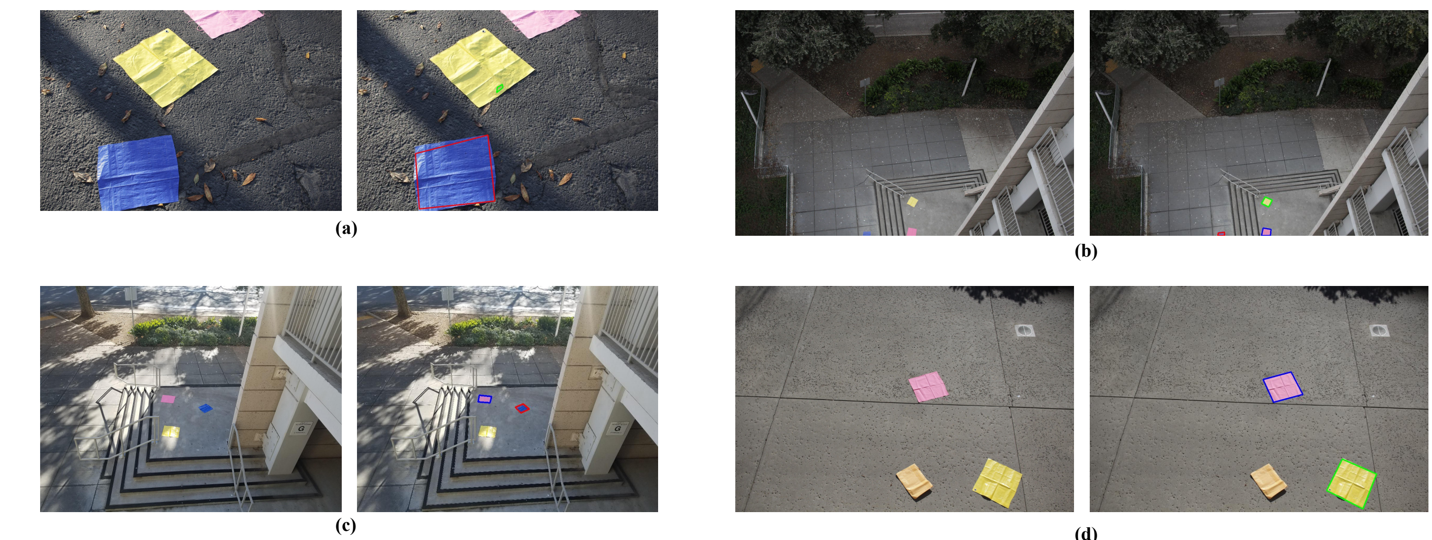
Figure 3: Sampling of pre- and post-processed images after the contour detection algorithm is run. Samples include: (a) Close-up (with off-screen target and varied lighting), (b) Large distance ~60 ft. (with off-screen target), (c) Midrange ~20 ft. (with varied lighting), (d) Confusing objects (with one missing target)
